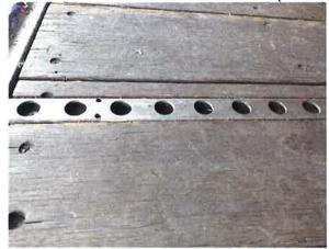
B. Aluminum Floor. Shows INCORRECT/wrong placement of "F" Track; should NOT be below floor level.
